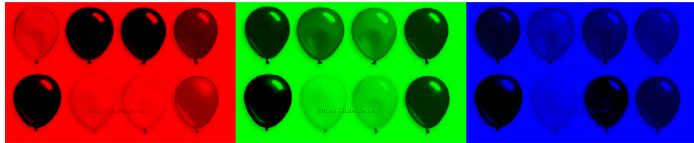
RED - GREEN - BLUE: R, G or B pixel = 0 is black, pixel = 255 is bright R, G or B
