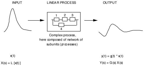
The overall transfer function (or the overall unit impulse reponse) can be determined from the transfer functions (or the unit impulse responses) of the subunits. For the process shown here:
